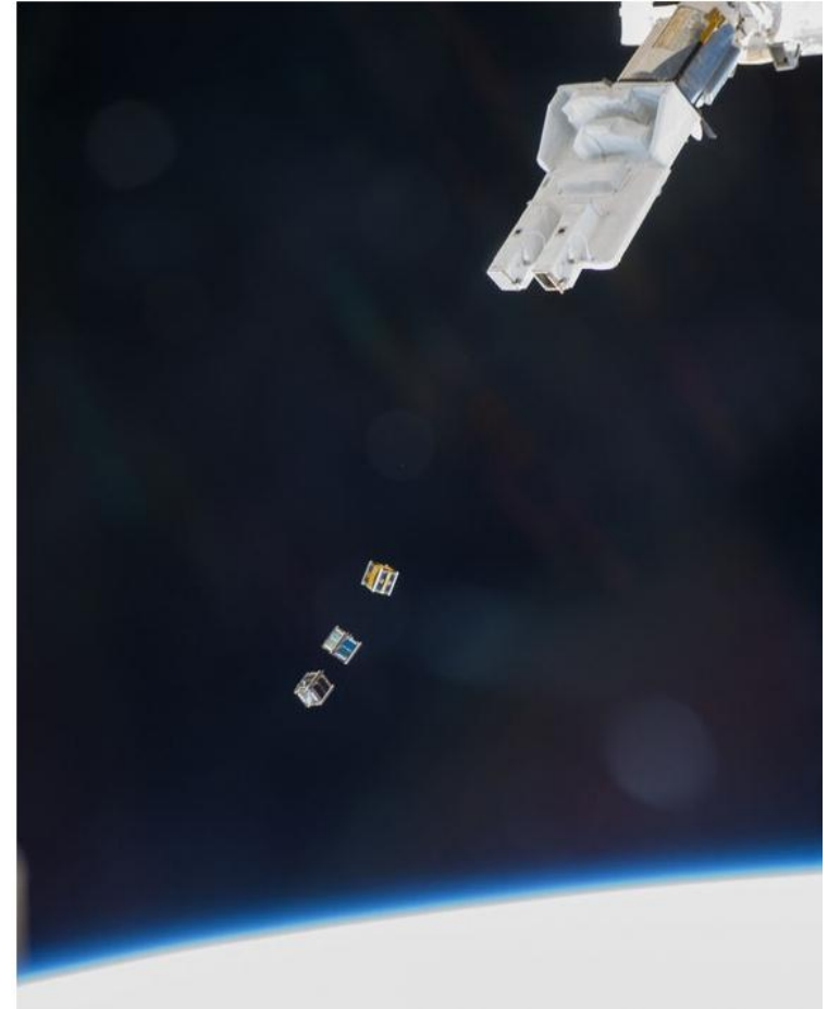
The International Space Station (ISS) releases three nanosatellites on November 19th, 2013 (source: NASA)
