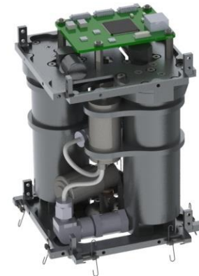
LituanicaSAT-2 visualization (Above) CubeSat propulsion system to be tested on LituanicaSAT-2 (Below)
